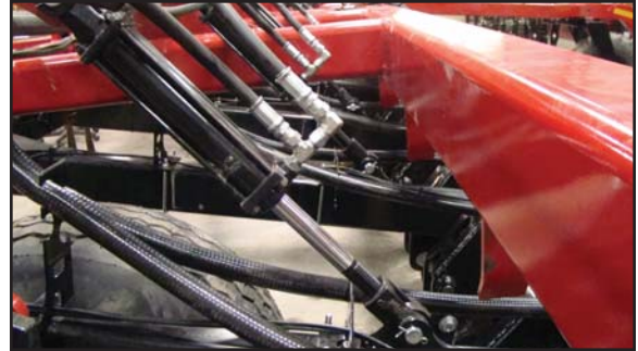
Down pressure cylinders
