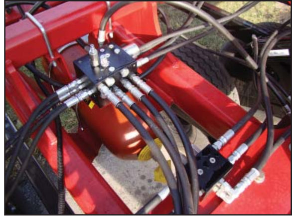
Flow divider valve lower right in photo
