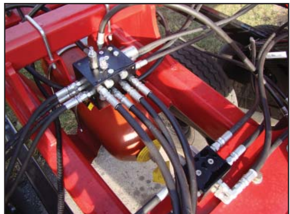
Accumulator and control valve
