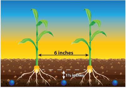
Optimal row width and fertilizer placement with the Single Disc Drill can give you a yield advantage vs. broadcast applications. Mid-row banding places starter fertilizer 3 inches from the plant row and up to 1½ inches below the seed, so as the plant grows, the roots reach the fertilizer at the right time in their development.
