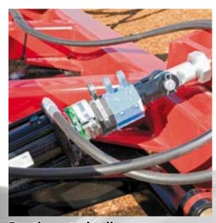
**Depth control collars** Depth control collars in the frame cylinders hold the frame exactly at the desired height.
