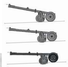
**Depth control adjustment** Height on the drill frame sets the depth of the row units. As the drill rises, the discs seed shallower. As the drill frame lowers, the discs seed deeper. Packer tires hold the discs precisely at seeding depth.
