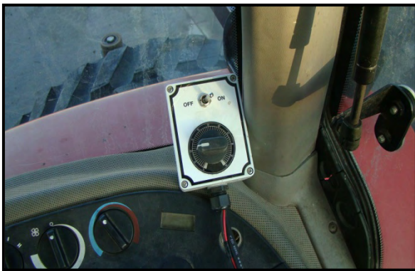
Down pressure control box in cab
