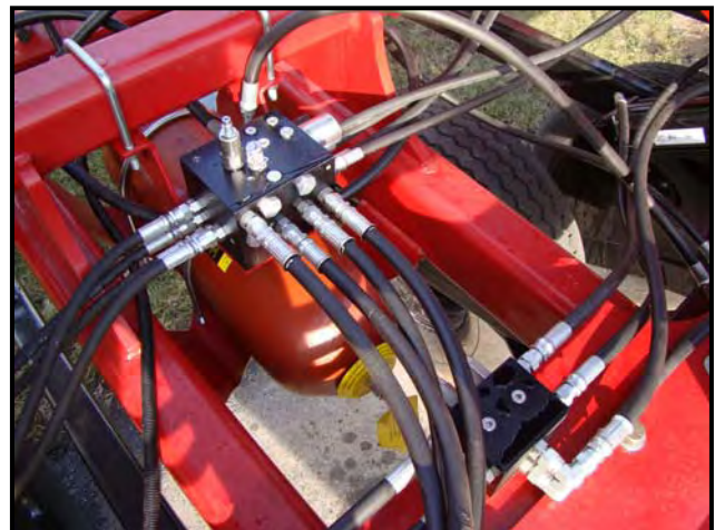
Flow divider valve lower right in photo
