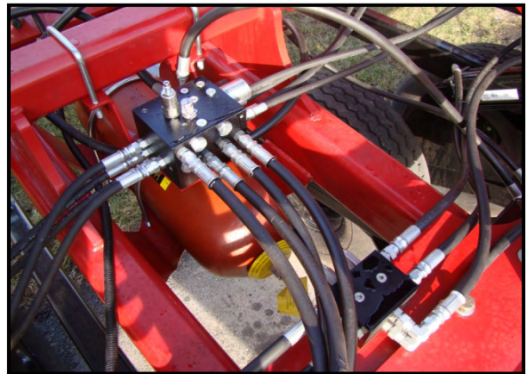
Accumulator and control valve
