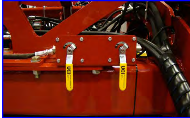
Lock out valves in closed position
