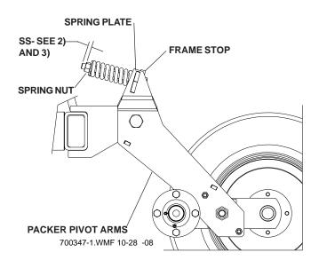
1) WITH THE MAIN FRAME LEVELTIGHTEN THE SPRING BOLT TO A (SS) DISTANCE OF APPROXIMATELY 3/8"-1/2" ON ALL THE MAIN FRAME PACKERS.
