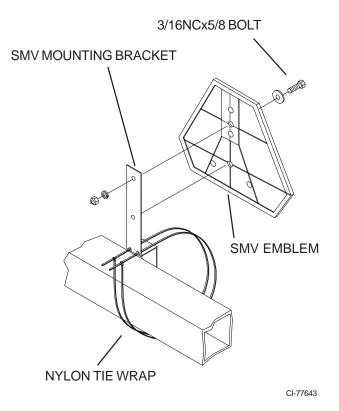
The bracket provided is designed to mount to numerous frame sizes and can be orientated in numerous positions to avoid interference with implement components.
