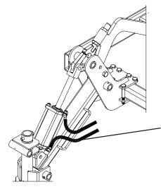
NOTE: CYLINDERS ON FRONT LIFT AXLES AND REAR PACKER LIFTS MUST BE MOUNTED WITH RODS UP AND PORTS TO THE SIDE. FAILURE TO ORIENTATE AS INDICATED CAN CAUSE PORT INTERFERENCE, CHECK FOR INTERFERENCE BEFORE AND WHILE ACTIVATING ALL CYLINDERS.
