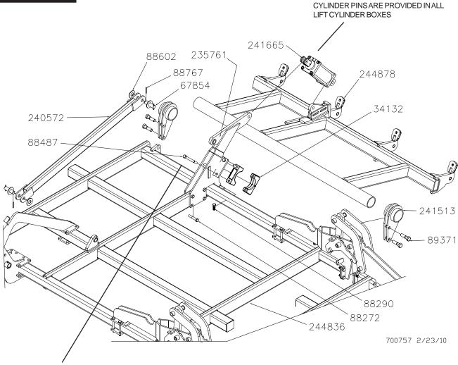
DO NOT OVERTIGHTEN 88487 BOLTS WHICH CAN CRACK 34132 BEARING CAPS
