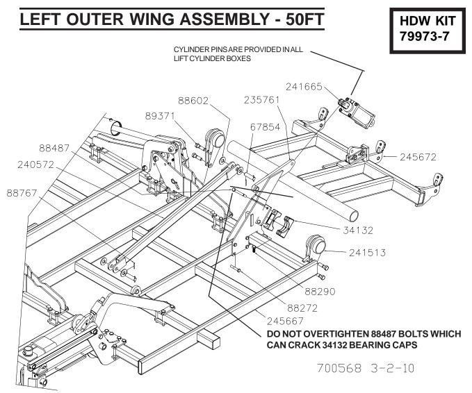
UNLESS SPECIFIED, ALL HARDWARE IS SECURED WITH MATCHING LOCK NUTS
