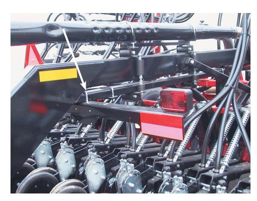
Bracket attaches with u-bolt to rear hitch. Note the light and decal placement.
