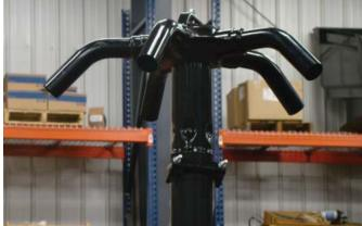
Position the outlets as shown on diagram. Hoses are precut to connect to secondary manifolds. Use the two longest hoses on the outside manifolds and the rest of the hoses on the other manifolds.
