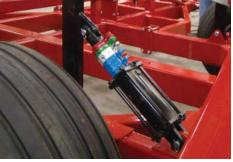
Install wing lift cylinders and hoses. Pin the base end of the cylinders to the main frame with cylinder pins provided. Remove plugs from cylinders. Pull cylinder rods out as far as possible.
