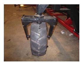
NOTE: ONLY TIGHTEN AXLE NUT UNTIL A SMALL RESISTANCE IS FELT WHEN TURNING WHEEL. BEARING FAILURE WILL RESULT IF OVER TIGHTENED.
