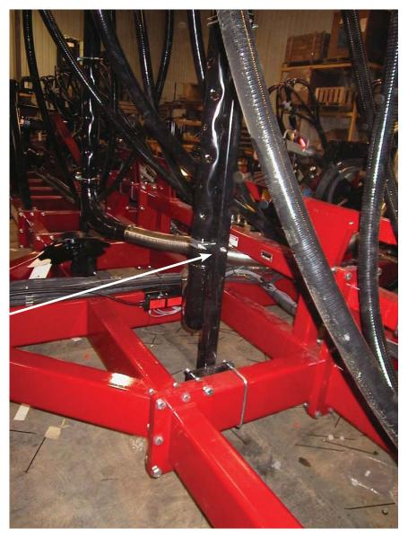
Offset manifolds about 2-inches in height to make it easier to install the 4-inch flexible hoses.
