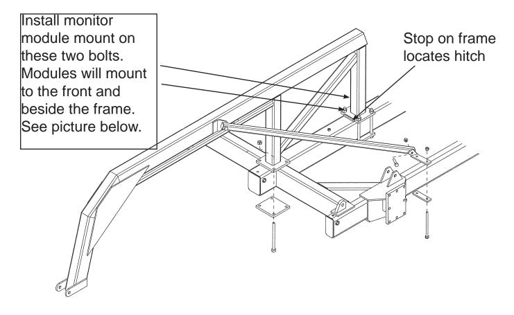
Install monitor module mount bracket to two of the hitch mount bolts as shown at right
