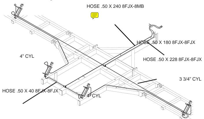
The cylinder decals indicate the size of the cylinder. The cylinder with a 40P in the number is the 4" and the one with 37P in the part number is the 3  $\frac{3}{4}$ ".
