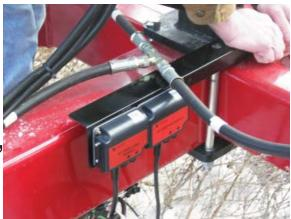
hitch mounting bolts. The modules plug into each other.
