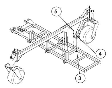
is mounted over the front rank of the wing frame. The rear (straight) leg is mounted over the  $4 \times 4$  front to rear frame brace member. This is the third front to rear brace from the end.
