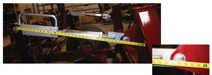
Attach caster frames to wing frames using <sup>3</sup>/<sub>4</sub>" u-bolts (Item 3) lock washers (Item 4) and nuts (Item 5).
