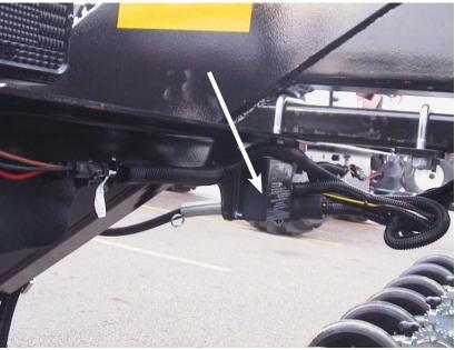
Mount the remote work switch on drill - it mounts to a bracket near the left main frame tire. (item A on diagram below) Connect a 4 meter minidin cable (small black monitor wire) to the work switch and plug it into any port on the bottom of the 3-load or flow module in the center of the drill. There are two locations on each module to plug in sensors (it doesn't matter which one you use).
