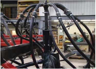
manifold. Continue connecting manifolds until all sensors are connected. Connect the last sensor in line back to the module.
