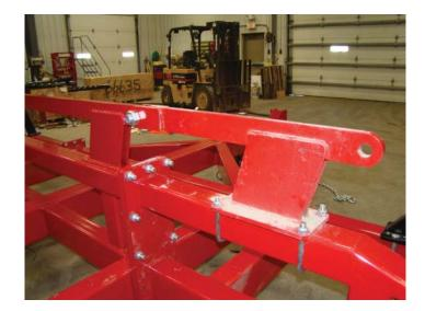
Mount row units. Measure out and mark opener locations per table below. Dimensions shown are from center of drill to center of row unit.
