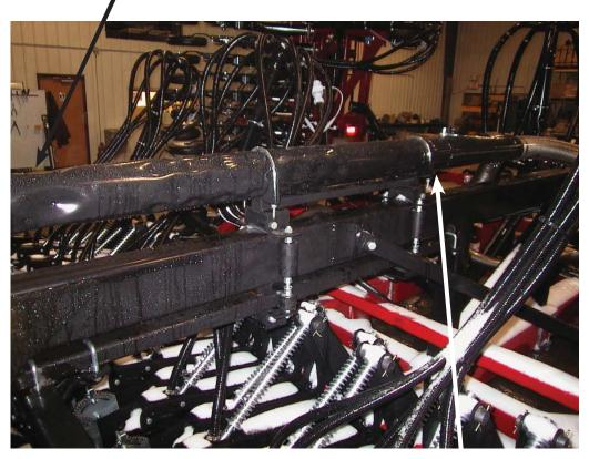
Front clamp close to front of straight section
