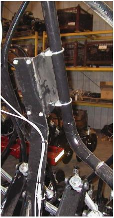
Connect 1 ¼" hoses between manifold outlets and disk openers. Fasten hoses with hose clamps. Cut all of the 1 ¼" hose to 75" long (191 mm).
