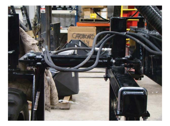
Hoses to cylinder mounted on marker beam (tip over cylinder)
