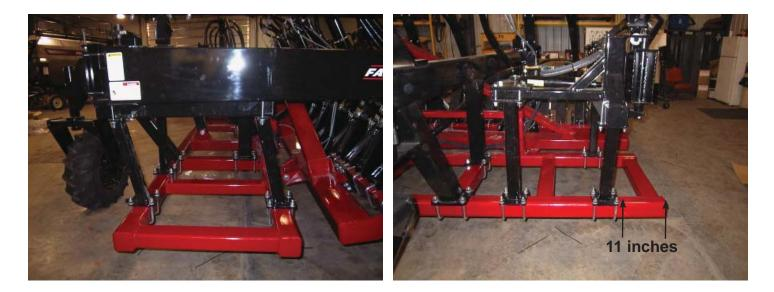
Mount straight stand just inside front to rear frame member. Attach with 5/8" u-bolts but do not tighten.
