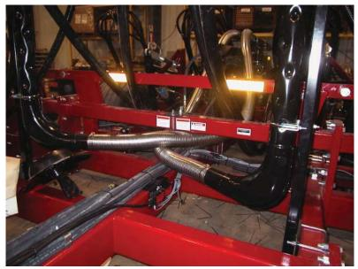
Mount two monitor modules to the main frame of the drill. The modules are labeled "Art module" and "three load module". Mount on module plate mounted to rear
