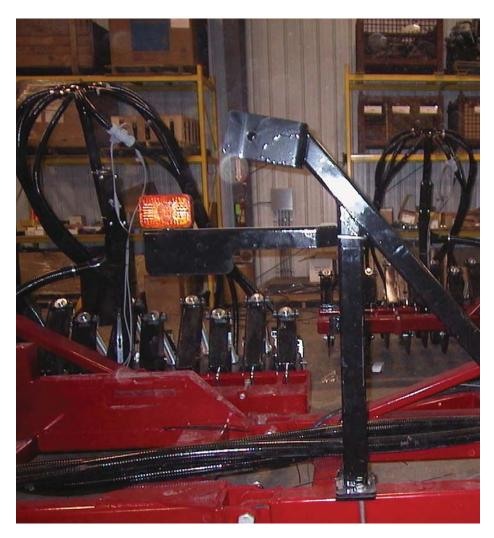
Note: Remember to tighten nuts on wing lock towers.
