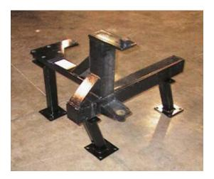
Install markers beams onto main mount with 1 <sup>1</sup>/<sub>4</sub>" pins and secure with 3/8" bolt and locknut.
