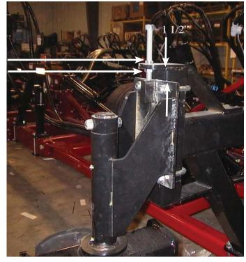
of mounting plate. Mount assembled caster using <sup>3</sup>/<sub>4</sub>" u-bolt (Item 3) lock washers (Item 5) and nuts (Item 4).
