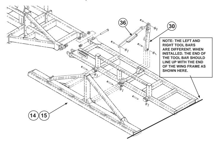
End of tool bar is in line with the end of wing frame when installed on correct side.
