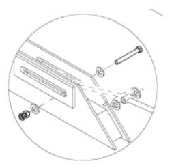
Connect rod end of cylinder into slotted hole on wing frame according to detail above. Flat washers are used on each side of each slot as shown. **Tighten nut only until it is close to slotted hole**. **Do not clamp bolt onto wing frame**. It has to be loose to slide freely. Use the jam nut to secure the nut.
