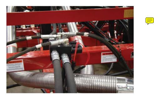
Connect the <sup>3</sup>⁄<sub>4</sub> hydraulic hoses to the front and rear of the valve. The hose that connects to the "P" port needs to be the hose that connects to the diverter on the air seeder tank.
