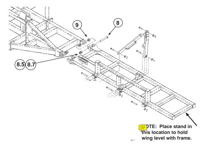
Attach wing frames to main frame with 1 ¼" x 10" bolts (Item 8). Each bolt is secured with a regular nut and a narrower jam nut (Items 8.5 and 8.7). Bolts should only be tightened until there is no side to side play. Do not tighten against ears. Tighten jam nut securely against regular nut.
