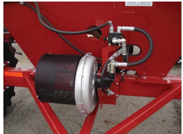
The blower and associated hydraulics
