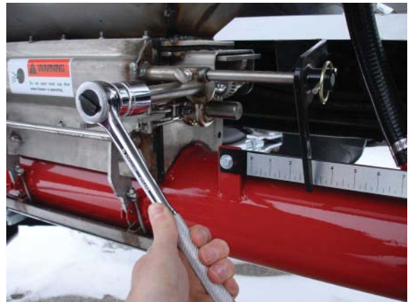
Adjusting the Meter Gate
