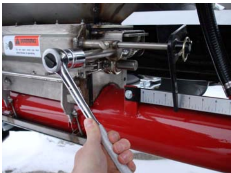
Adjusting the Meter Gate
