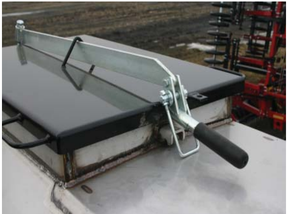
Lid and latch with toggle u-bolt adjustment
