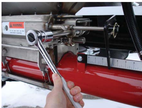
Adjusting the Meter Gate
