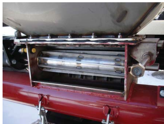
The meter with door removed
