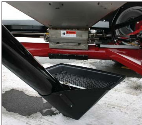
Placing the hopper under the meter
