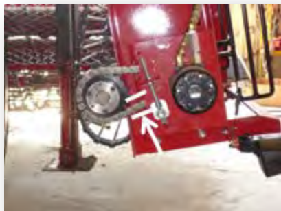
Figure 62: Reduction Chain Tension
