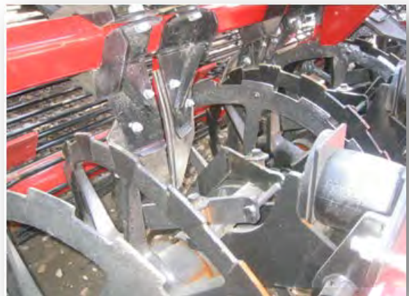
Figure 82: Lifter Strut and Paddle Cleaning
