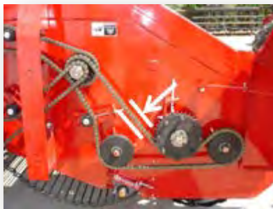
Figure 61: Paddle Shaft Chain Tension
