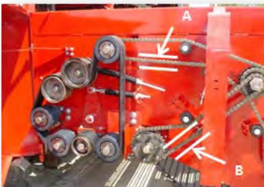
Figure 65: Drive and Apron Shaft Chain
