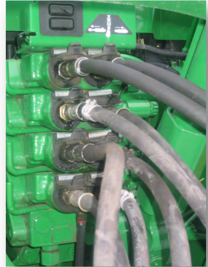
Figure 18: Attaching Hydraulic Lines
