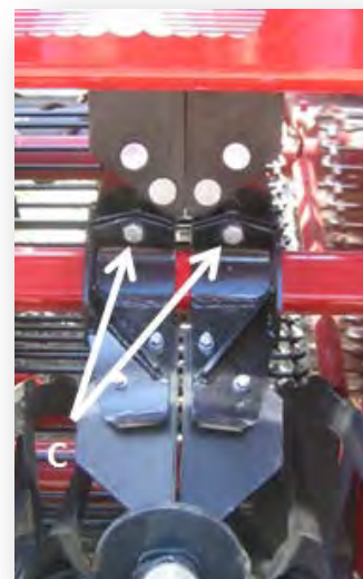
Figure 51: Rubber Paddle Adjustment
