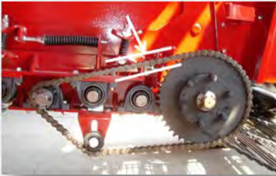
Figure 63: Jump Chain Tension
