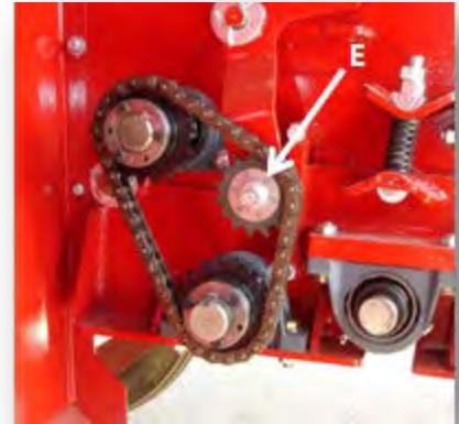
Figure 69: Grabroll Drive Chain Adjustment
