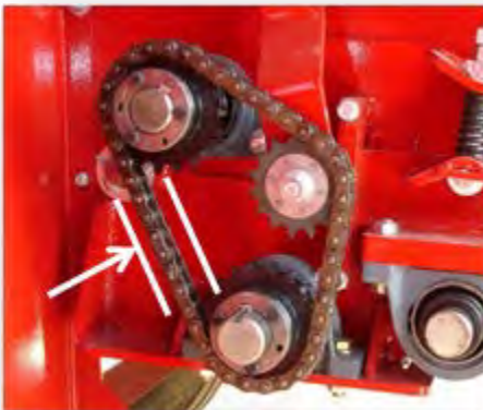
Figure 64: Grabroll Bed Chain Tension
