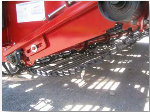
Figure 84: Apron Shaft Cleaning
