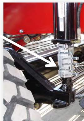
Figure 23: Manual Leveling Adjustment
