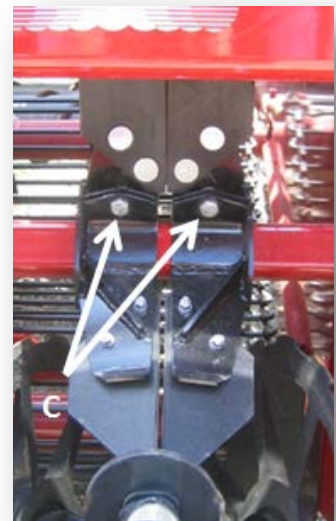
Figure 51: Rubber Paddle Adjustment
