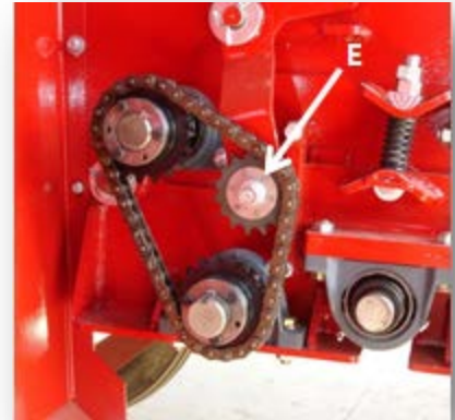
Figure 69: Grabroll Drive Chain Adjustment
