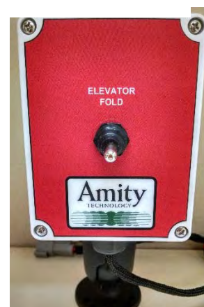
Figure 4-2: Elevator Control Box
