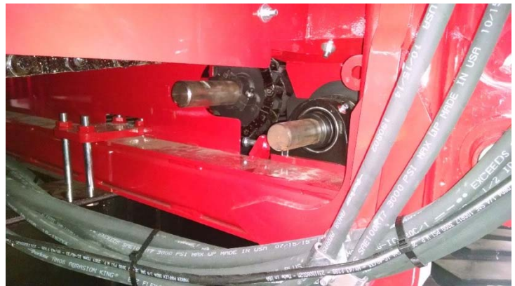
Figure 9-2: Feed Roller and Center Floor Drive Shafts
