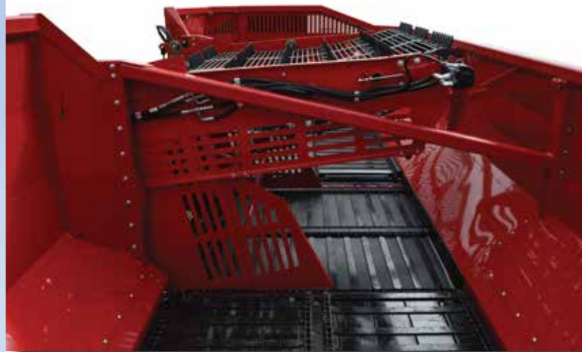
The unloading elevator fold inside the sugar beet cart for narrower transport.
