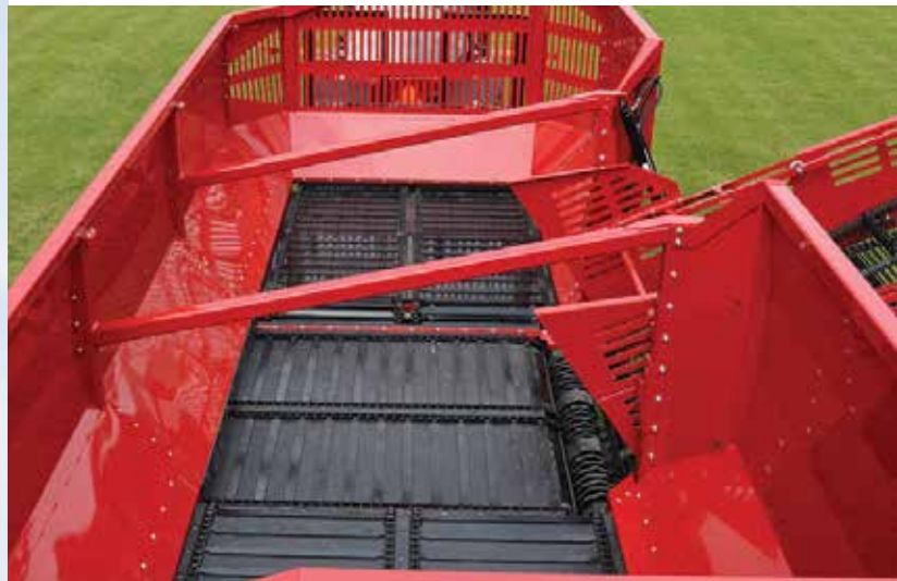
Solid floor and drag chains eliminate unacceptable beet damage in dry conditions.
