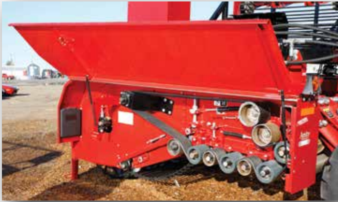
Shield with gas shocks provides easy access to working components.
