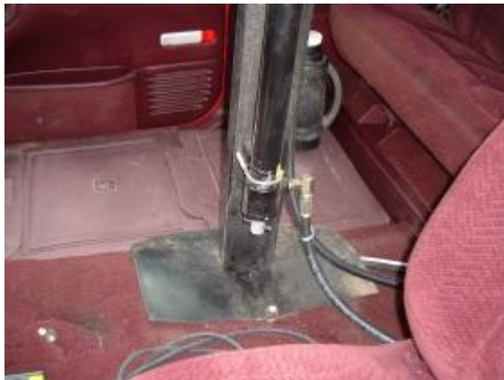
Inside mounting example, rubber dust seal.
