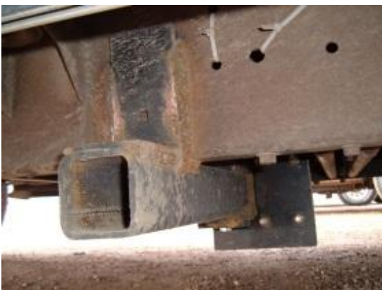
Cross member can be bolted or welded to frame.
