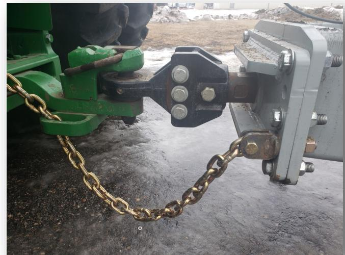
Figure 5-2: Attaching Harvester to Tractor Drawbar
