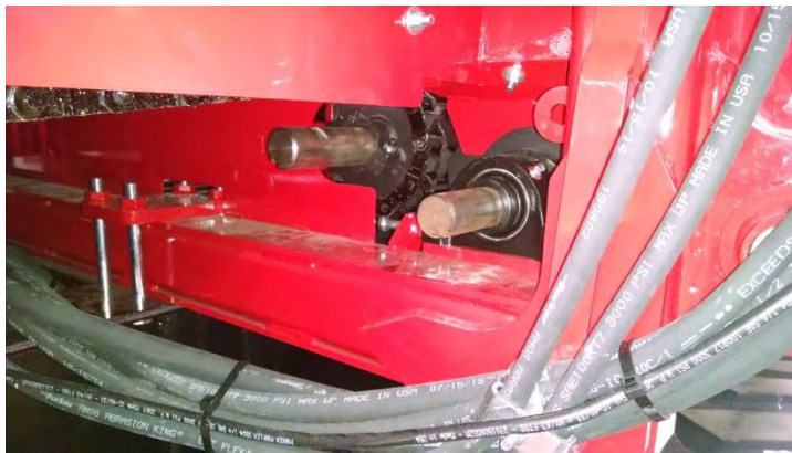
Figure 9-2: Feed Roller and Center Floor Drive Shafts
