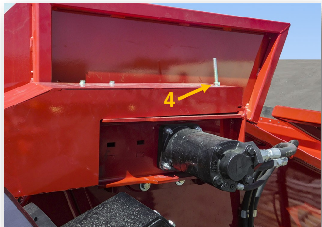
Figure 8-27: Drive Motor Chain Tension
