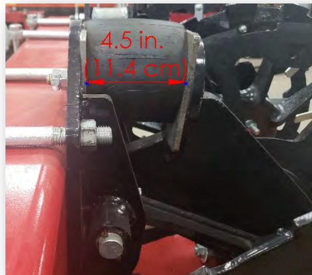
Figure 7-8: Rock Cushion Tension
