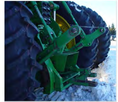
Figure 4-1: Fully Raised Three-Point Hitch
