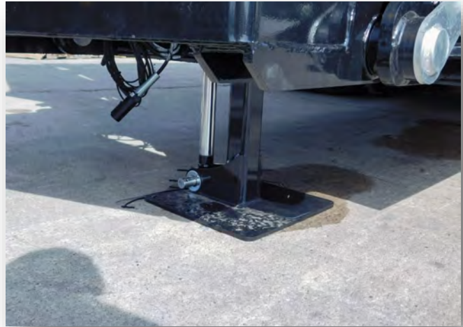
Figure 5-1: Hydraulic Jack in Lowered Position
