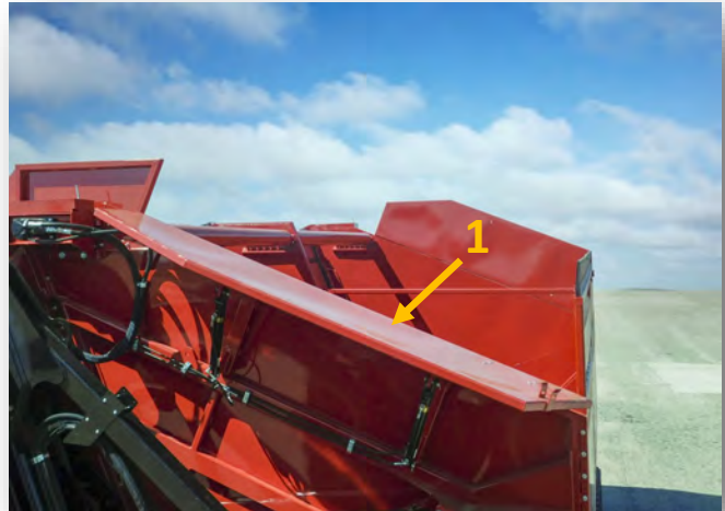
Figure 6-1: Front Top Gate in Lowered Position
