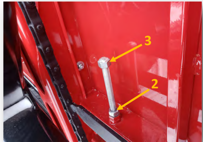
Figure 8-26: Unloading Chain Tension Adjusting Screw
