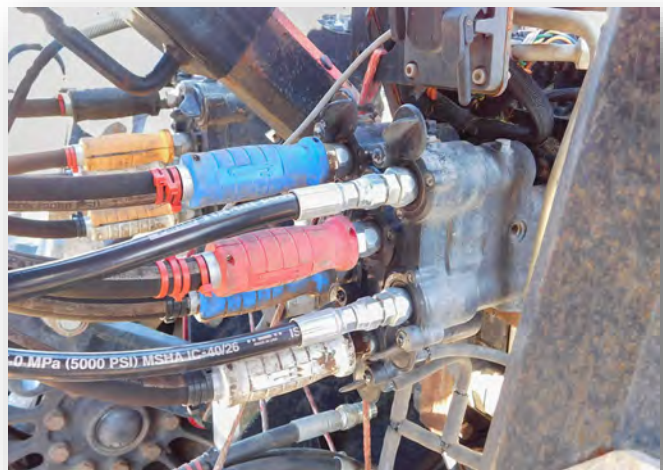
Figure 5-2: Attaching Hydraulic Hoses
