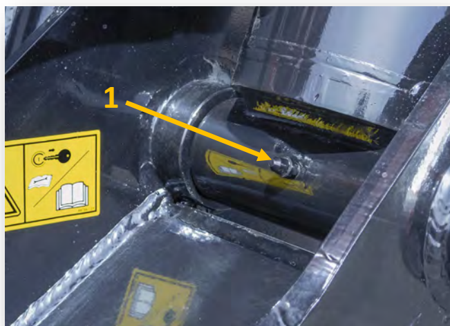
Figure 8-9: Rear Lift Cylinder Base End Fitting
