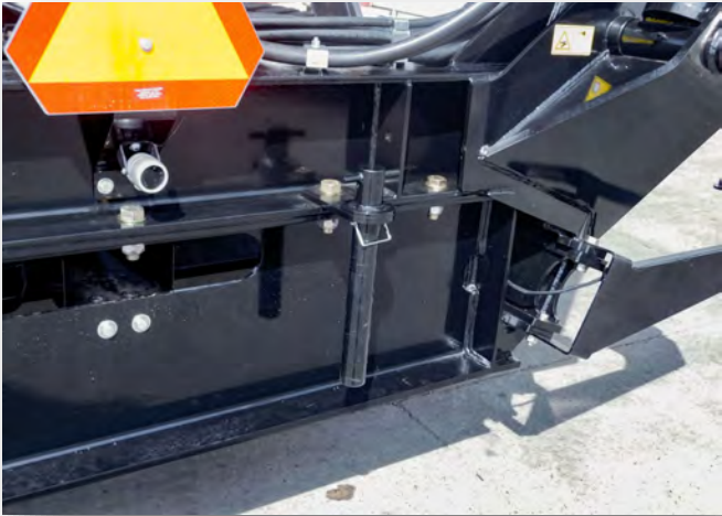
Figure 8-3: Tank Safety Pin Storage Location
