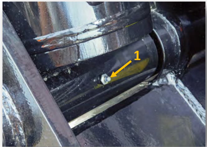
Figure 8-13: Front Lift Cylinder Base End Grease Fitting
