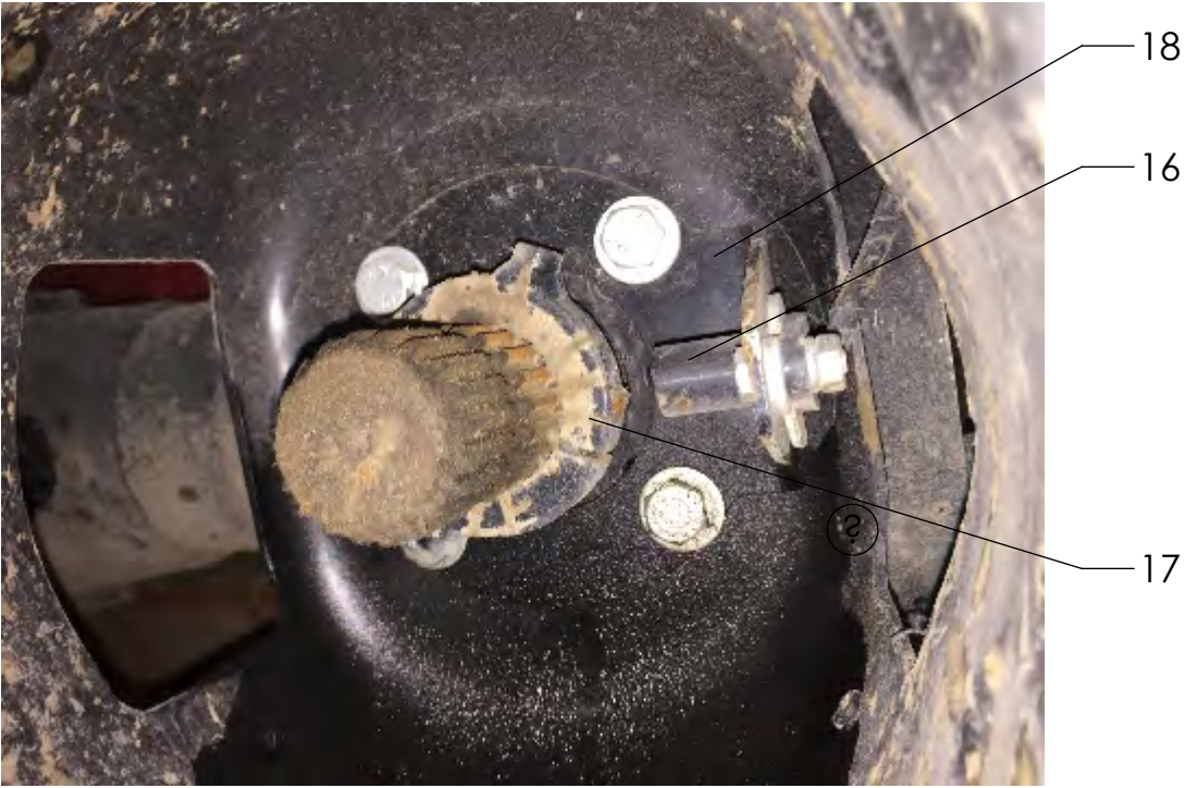
FIG. 1 - PTO SENSOR MOUNT
