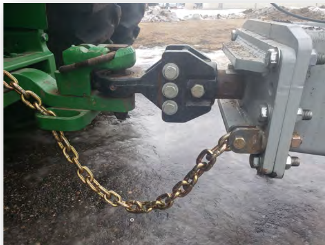
Figure 5-2: Attaching Defoliator to Tractor Drawbar
