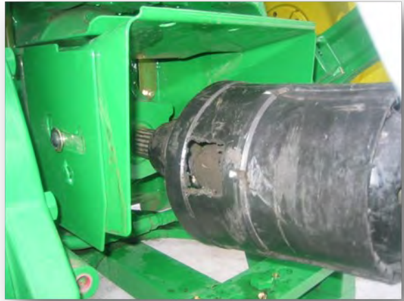
Figure 5-3: Attached PTO Driveline
