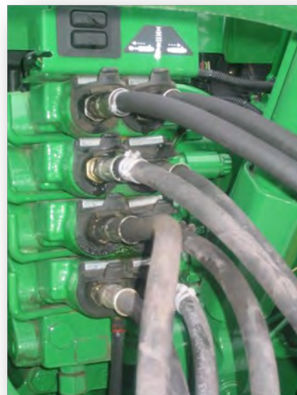
Figure 5-1: Attaching Hydraulic Lines
