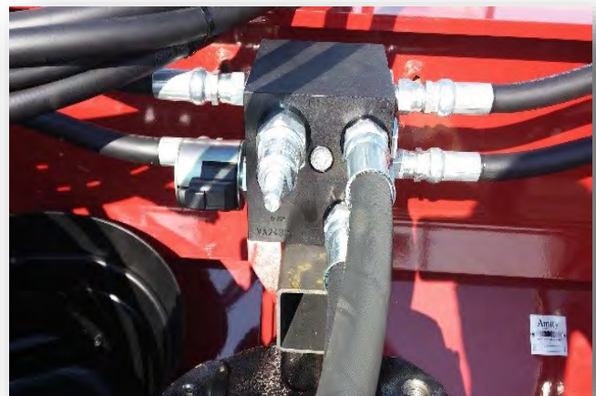
Figure 6-4: Floating Hitch Valve
