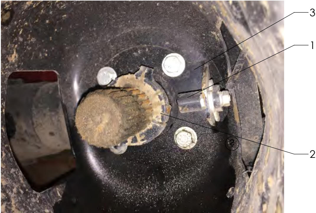
FIG. 1 - PTO SENSOR MOUNT
