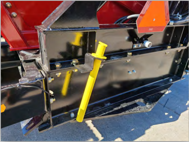
Figure 8-3: Tank Safety Pin Storage Location
