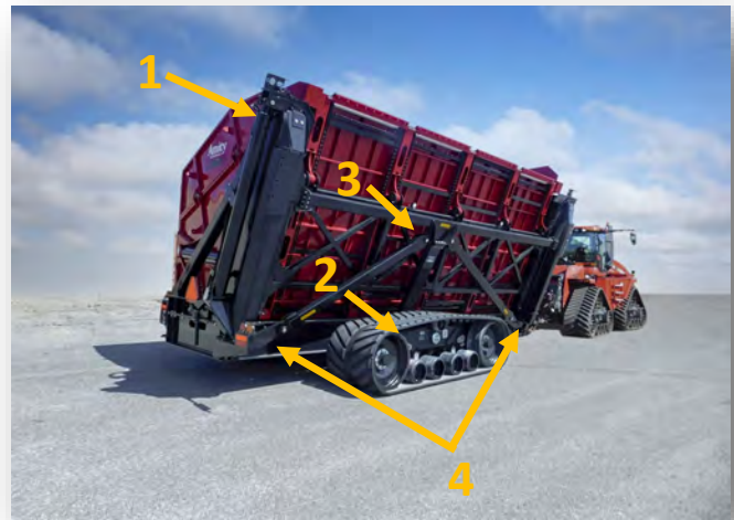
Figure 8-1: Areas of Debris Buildup
