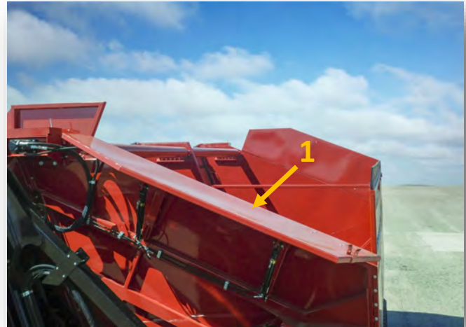
Figure 6-1: Front Top Gate in Lowered Position
