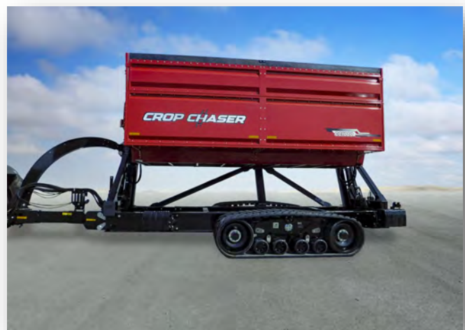
Figure 8-2: Tank Raised for Cleaning
