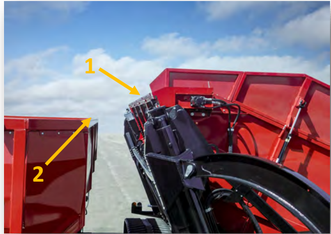
Figure 6-2: Tank Distance from Receiving Unit
