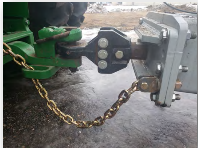
Figure 5-2: Attaching Defoliator to Tractor Drawbar
