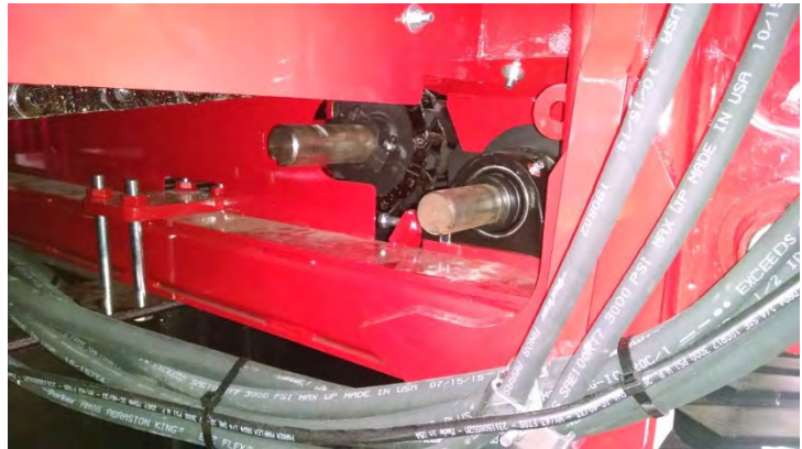
Figure 9-2: Feed Roller and Center Floor Drive Shafts
