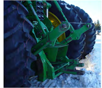
Figure 4-1: Fully Raised Three-Point Hitch
