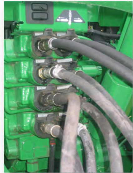
Figure 5-1: Attaching Hydraulic Lines
