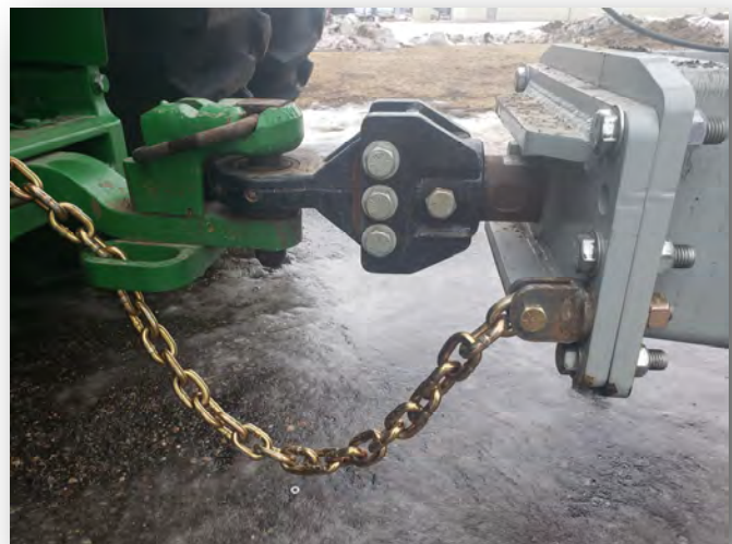
Figure 5-2: Attaching Cart to Tractor Drawbar
