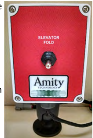
Figure 4-2: Elevator Control Box
