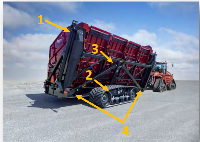
Figure 8-1: Areas of Debris Buildup
