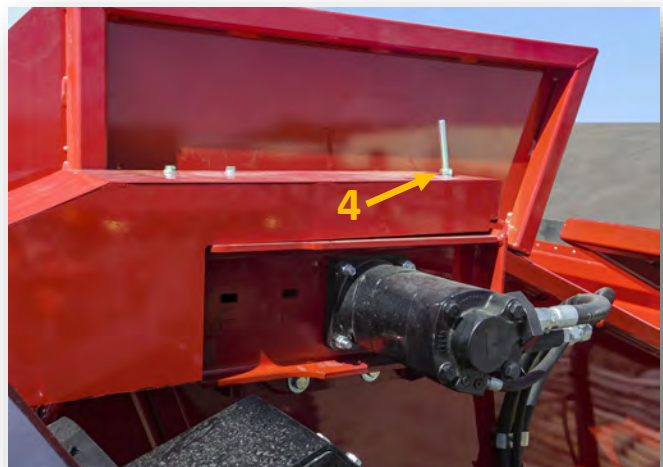
Figure 8-28: Drive Motor Chain Tension
