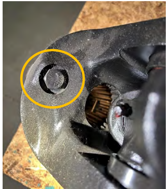
Figure 12-7: Shear Bolt Orientation—Bolt Head
