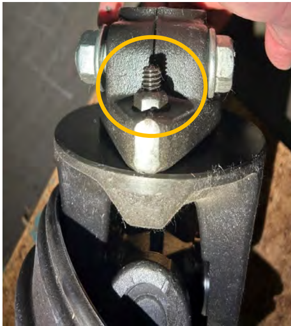
Figure 12-6: Shear Bolt Orientation—Lock Nut
