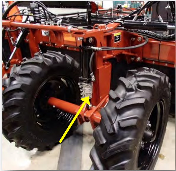
Figure 7-2: Rear Strut Height Adjustment
