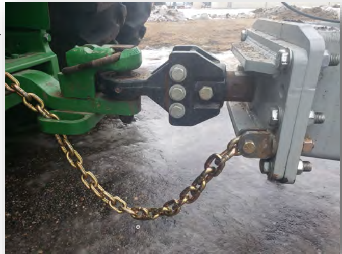
Figure 5-2: Attaching Defoliator to Tractor Drawbar
