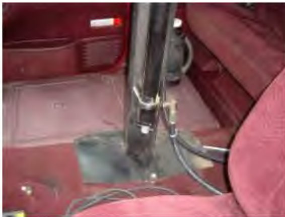
Inside mounting example, rubber dust seal.
