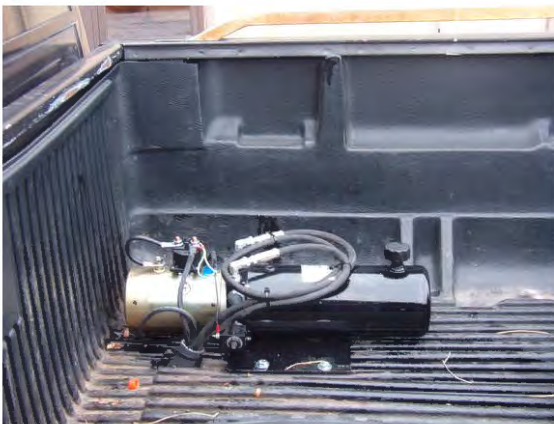
Power unit mounted in box
