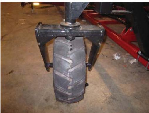
Tire should be in center of caster. If not, it is mounted backwards on the hub.
