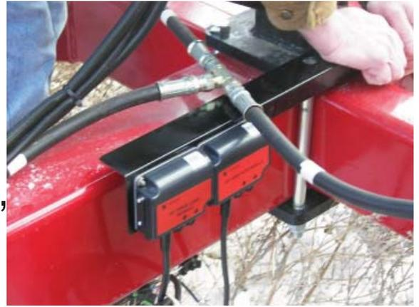
Connect the longest large black monitor cable (5 meter) to the front of the modules and route to the front of the drill. Connect a 3 meter to the rear of the modules and route to hitch point at rear of drill.
