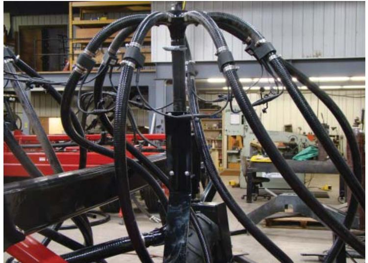
Connect the sensor on the first manifold to the sensor on the next manifold. Continue connecting manifolds until all sensors are connected. Connect the last sensor in line back to the module.
