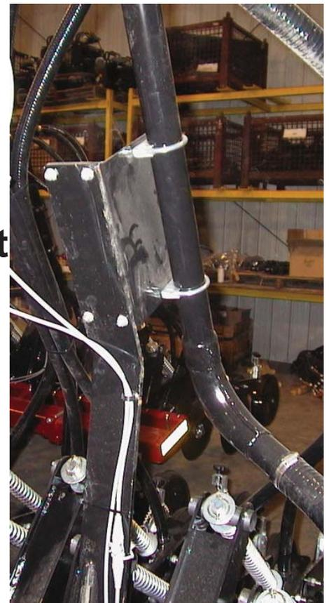
Connect 1 ¼” hoses between manifold outlets and disk openers. Fasten hoses with hose clamps. Cut all of the 1 ¼” hose to 75” long (191 mm).
