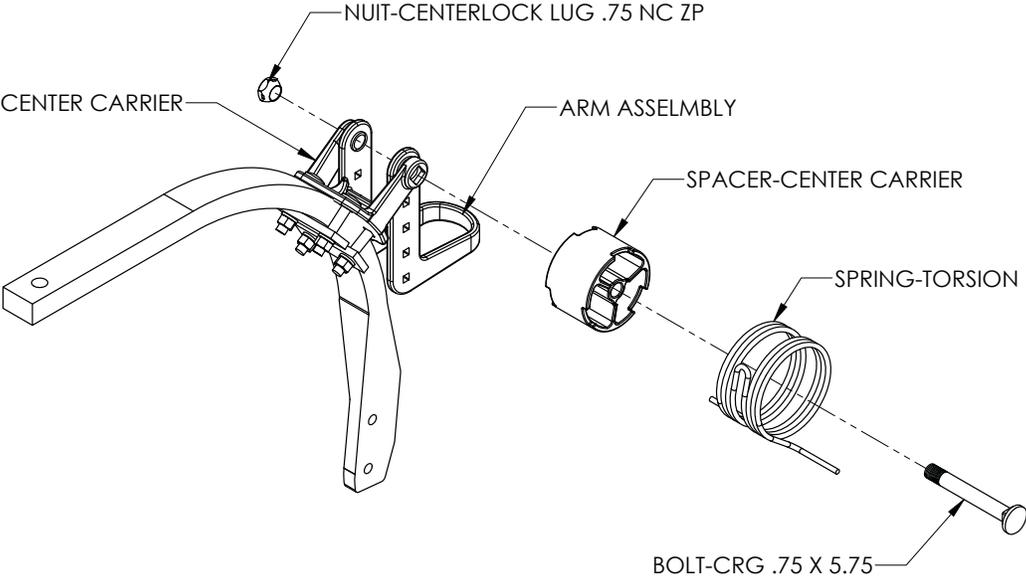
Adjust the Center Carrier until the Disc Leveler Torsion Spring is 0.25" from shank spring as shown. Finish tightening the four carriage bolts to the shank.
