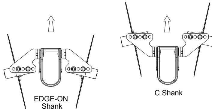
Assemble the Arm Assembly as shown, ensuring vertical height is 1"-3" above sweep
